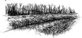
Swales are designed by taking into account road slope, the volume of water needed to be collected and filtered and the placement and size of driveway culverts. Swales can also be lined with grass or stone.
